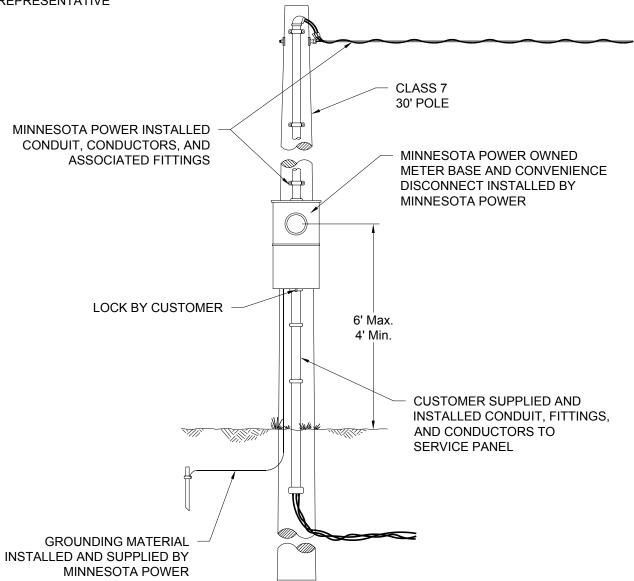
"METER POLE INSTALLATION CAN BE ACCOMPLISHED ON SELECT COMPANY POLES. ANY DESIGN MUST ASSURE THAT THE POLE IS TRUCK ACCESSIBLE AND "CLEAR" OF OBSTRUCTING ELECTRIC EQUIPMENT. EXAMPLES OF NON-OBSTRUCTING EQUIPMENT WOULD INCLUDE CONDUCTORS, CROSS-ARMS, TRANSFORMERS, DOWN GUYS AND LEASE LIGHTING. POLES SUPPORTING SWITCHES, CAPACITOR BANKS, REGULATORS OR PRIMARY RISERS WILL NOT BE USED FOR METER POLE INSTALLATIONS."
