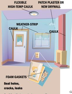
Anything that penetrates your walls or ceilings is a potential location for an air leak. Gaps around windows, doors, fireplaces, electrical boxes—even cracks in plaster—can allow air to move between the inside and outside of your house. Seal them up with caulk, weather-stripping, or plaster. And foam gaskets on outlets and switches can increase comfort, avoiding unnecessary energy use.
