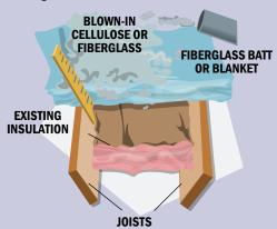
Insulation slows the heat flow through a building's envelope. It works year-round to make your home more comfortable and energy efficient. In the winter it slows heat loss and in the summer reduces heat gain and helps keep your home cool.
