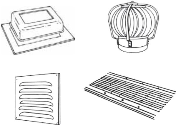
Here's the rule of thumb for attic ventilation: If there is a vapor barrier, one square foot of outside ventilation is needed for each 300 square feet of attic floor. If there is no vapor barrier and the roof has less than a three-foot rise from eave to peak, one square foot of ventilation is needed for every 150 square feet of attic floor.
