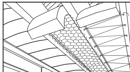
attached, to the underside of the floors. The vapor barrier goes on the “winter-warm” side of the insulation—in other words, toward the inside of the house.
