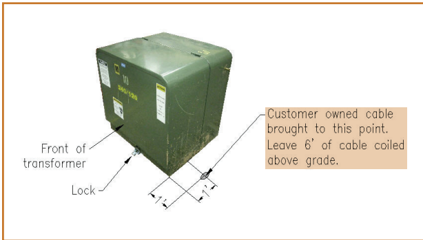
Front side of pad-mounted transformer with lock
