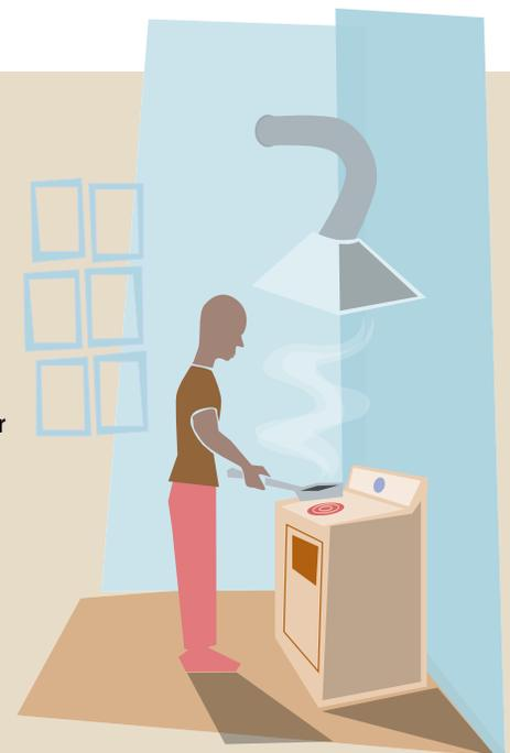
good job of removing smoke, dust, and other contaminants very quickly. However, their very power can lead to problems with inadequate air supply and they usually require additional make-up air.
